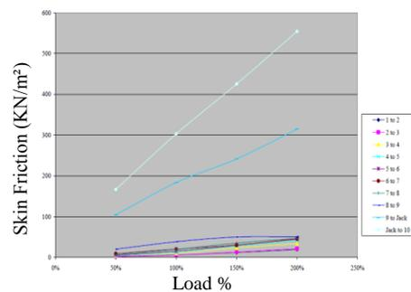
Figure 8. Skin Friction vs Load (%).
