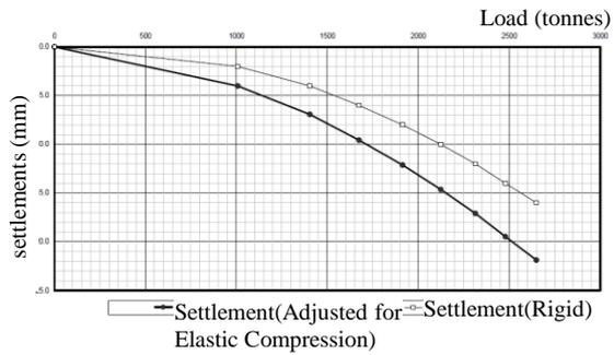
Figure 7. Settlements vs Load.
