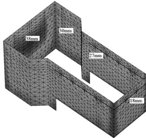
Figure 5. Diaphragm Wall Displacement With 3D Model Calculation
