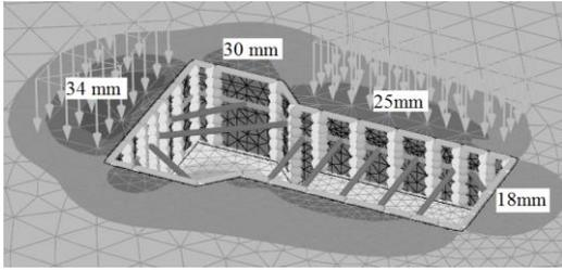
Figure 6. Surface Settlements With 3D Model Calculation
